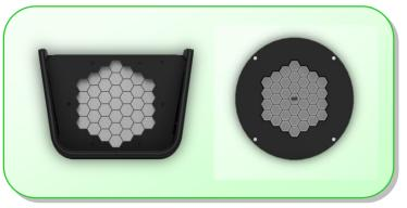
534 for conventional and high-speed vehicles when using 36 plastic customised optical elements. The lamp is fitted with 36 white LEDs for use in marker lamp mode and 36 red LEDs for use in tail lamp mode, with each colour controlled by a separate driver. LED drivers also perform diagnostics of the LEDs and indicate any fault states on the diagnostic relay output. The luminous intensity of the LED-based MTL04 lamp is adjustable to several levels.
